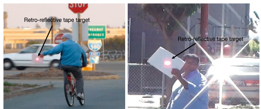
Fig. 7 Outdoor tracking of targets moving on a bike, and in direct sunlight. Targets are red due to the tracking laser beam centering on them. At the shown distances of \sim 80 \text{ m} , the beam size is nearly identical to the target size of 5 cm.
