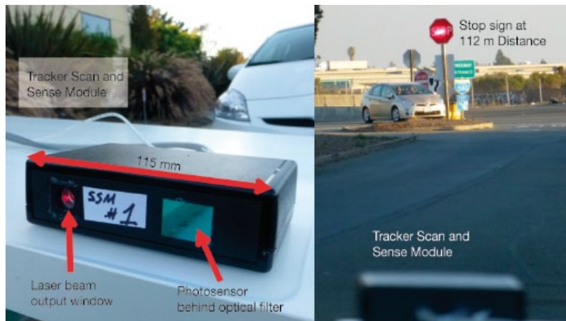
Fig. 6 Scan and Sense Module (SSM) for longer range outdoor applications. A stop sign with inherent retro-reflective properties acts as a highly attractive target to the system, even at 112 m distance and is therefore illuminated by the 660 nm red laser beam.
