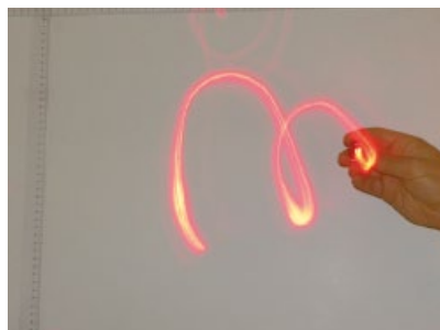
Fig. 3 Photographs of a corner-cube retro-reflector (CCR) and retro-reflective tape being tracked by the MEMSEye system. The red glow in the images is caused by the red laser beam which is directed by the MEMS mirror to track the objects. Fast hand movement in the left image and an extended exposure time of the photograph shows the trail of target and laser beam positions.
