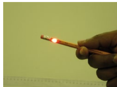
Fig. 3 Photographs of a corner-cube retro-reflector (CCR) and retro-reflective tape being tracked by the MEMSEye system. The red glow in the images is caused by the red laser beam which is directed by the MEMS mirror to track the objects. Fast hand movement in the left image and an extended exposure time of the photograph shows the trail of target and laser beam positions.
