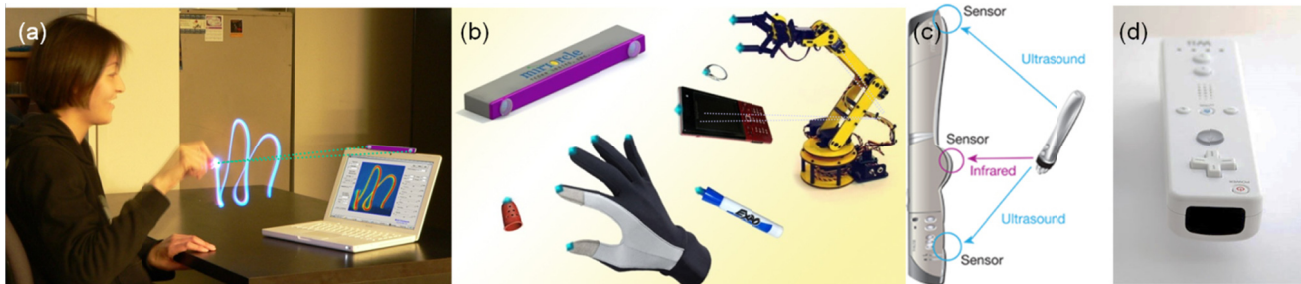
Figure 1. Depiction of our project’s long-term goal – a sensor unit with two optical-tracking apertures measure 3D position of a remote object, shown here as a small glowing blue LED. In (a), the sensor unit is mounted on top of a laptop’s monitor and a user is running a 3D application. In (b), we depict various possible system uses based on where we attach the small tracking targets. For example, robot’s end effector position is monitored. (c) Mimio’s interactive electronic white board kit allows hand written materials and drawings on whiteboard to be recorded electronically in color. (d) Nintendo’s Wii remote senses the user’s motion and use it to interact with a game.
