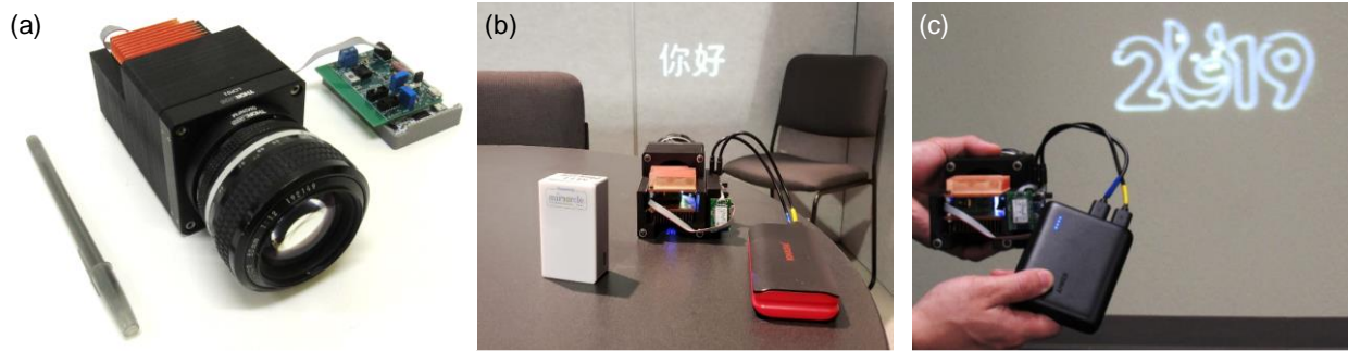
Figure 11. (a) The Programmable Light System with a Nikon 50mm camera lens for projection, and the OCCIE MEMS controller with a Bluetooth module and a high current (>2A) laser driver, (b) the latest PLS module displaying “Ni Hao” Chinese characters, (c) the PLS white light projection system displaying a vector graphic, with a light-weight and compact design, and battery operated for easy mounting and demonstration of technology.
