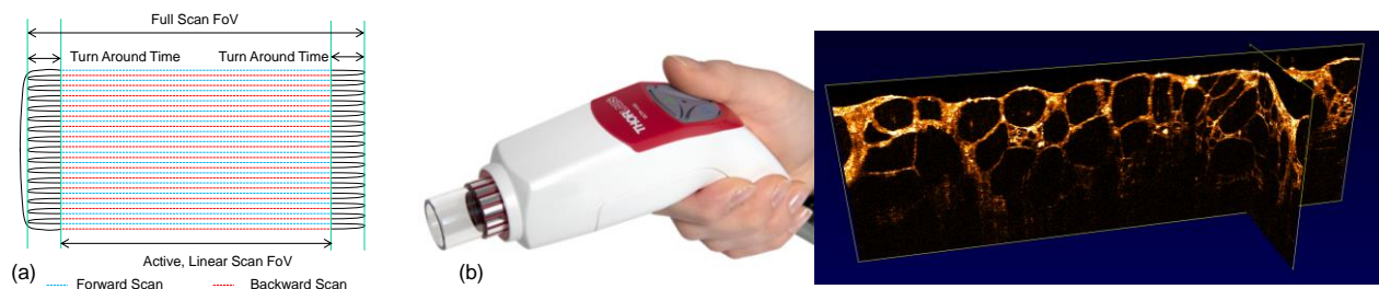
Figure 3. (a) Example of a linear raster scan that can be optimized for a MEMS mirror by training the device in iterative learning, and be driven in open loop, (b) example of a bio-medical imaging handheld scanner that uses a gimbal-less, dual-axis MEMS mirror, Thorlabs part OCTH-900.
