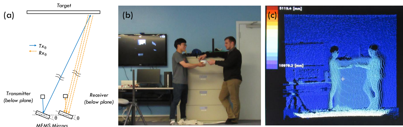
Figure 7. (a) The SyMPL 3D LiDAR architecture uses two MEMS mirrors to direct the transmitted beam and the receiver's aperture simultaneously, to the same region. (b) An image of the scene addressed by the SyMPL 3D LiDAR. (c) The point cloud generated of the scene using SyMPL 3D LiDAR
