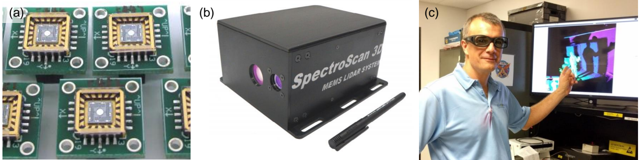
Figure 1. MEMS mirror based scanning LiDAR systems: a) MEMS mirrors of 1.2mm diameter (A3I12.2-1200AL) packaged in 9mm x 9mm wide ceramic carrier in connectorized PCBA form for easy mounting in prototype Scan Modules, b) MEMS LiDAR SYSTEM "SpectroScan 3D" from Boeing Spectrolab [10], c) Lead author is testing a similar MEMS LiDAR system developed at NASA Goddard [15].
