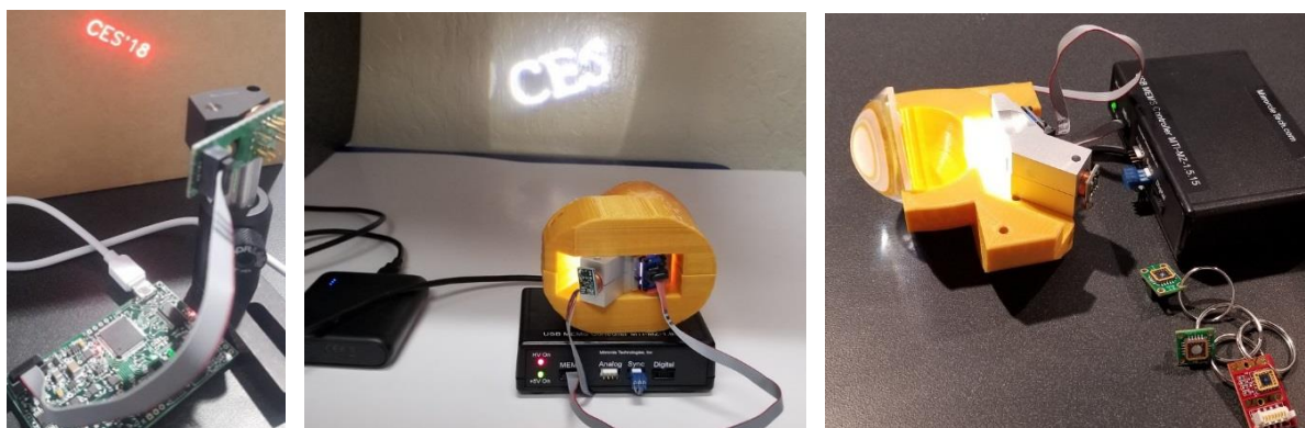
Figure 2. Demos from CES2018 in Las Vegas, NV. (a) a prototype Playzer Scan Module PZEK-01R demonstrates the compact opto-mechanical setup of a MEMS mirror laser and optics with a 40° FoV and the compact USB battery powered OCCIE 1.1 MEMS controller, (b) PLS-01 powered by a USB battery, running from the USB-SL MZ MEMS Controller with flashed content, (c) the PLS-01 with the cover off to show the MEMS mirror scan module, transmissive phosphor target and condenser lens.
