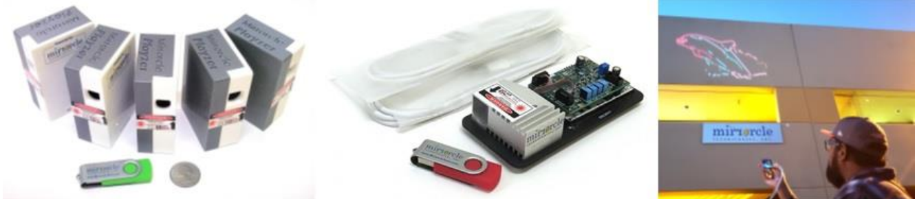
Figure 2. Mirrorcle Vector Graphics Laser Projectors (VGLP) Playzers (left) and the new RGB Playzer (development kit center and outdoor demonstration right).
