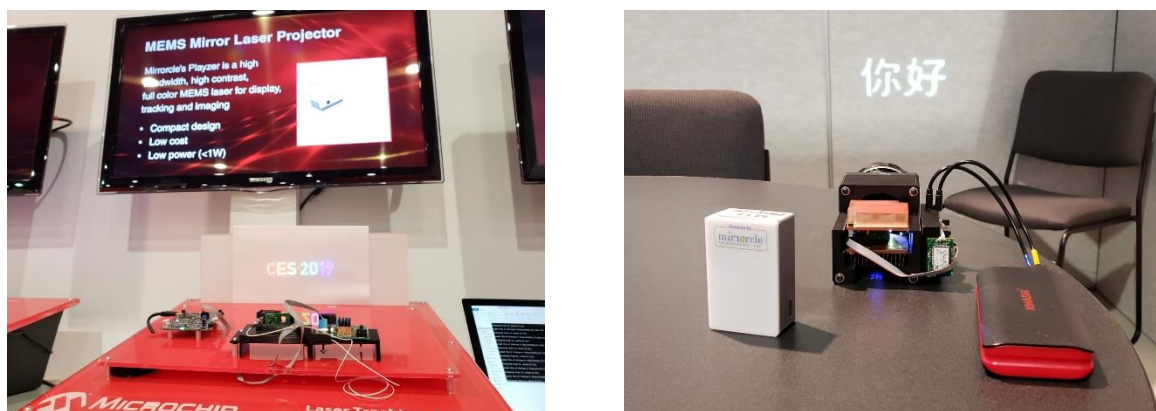
Figure 2. Mirrorcle Technologies' application demonstration examples at CES 2019 in Las Vegas, NV. (a) a Scan Module demonstrates the compact opto-mechanical setup of a MEMS mirror laser and optics with a 40° FoV and the compact USB battery powered OCCIE MEMS controller, (b) PLS powered by a USB battery displays a Chinese greeting in bright white light. The smaller white box contains a regular pocket-sized Playzer laser projector with a battery and wireless controller.
