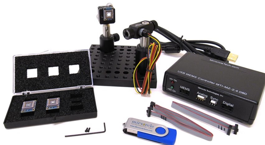
Figure 1. Mirrorcle Technologies' popular 'Standard Development Kit' containing 3 dual-axis MEMS mirrors, a versatile USB-SL MZ Controller, mounting accessories and the Mirrorcle Software Suite..
