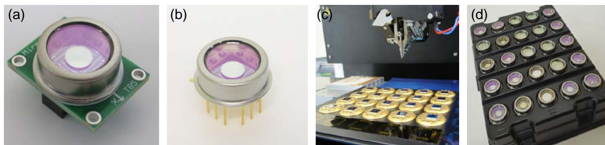
Figure 1. (a) MEMS Mirror (P/N: MEMS device A5L2.2-4600AL-TINYTO8.4-CAPSC2) in hermetic and connectorized package TINYTO8.4, (b) MEMS Mirror (P/N: A5L3.3-5000AL-TO8-CAPSC2) in a bare TO8 hermetic package, (c) MEMS Mirror automated assembly in Mirrorcle's facilities, (d) manufactured hermetically packaged devices for customer delivery.
