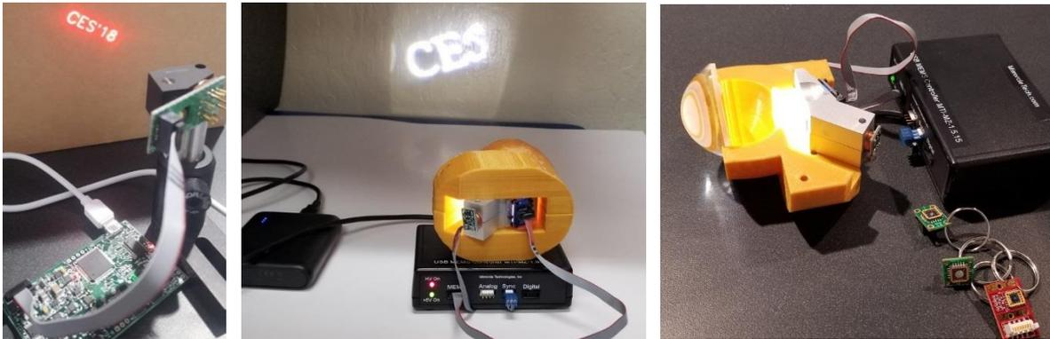
Figure 2. Playzer prototype with new USB Controller OCCIE 1.1 and new compact scan module (left). Programmable Light Source PLS-01 projecting white-light "CES" text (middle). Open PLS-01 module with MEMS-based scanner and integrated laser, phosphorous and optics. Also shown is the Mirrorcle USB-SL MZ controller powered by Microchip's PIC32MZ high voltage driver IC.
