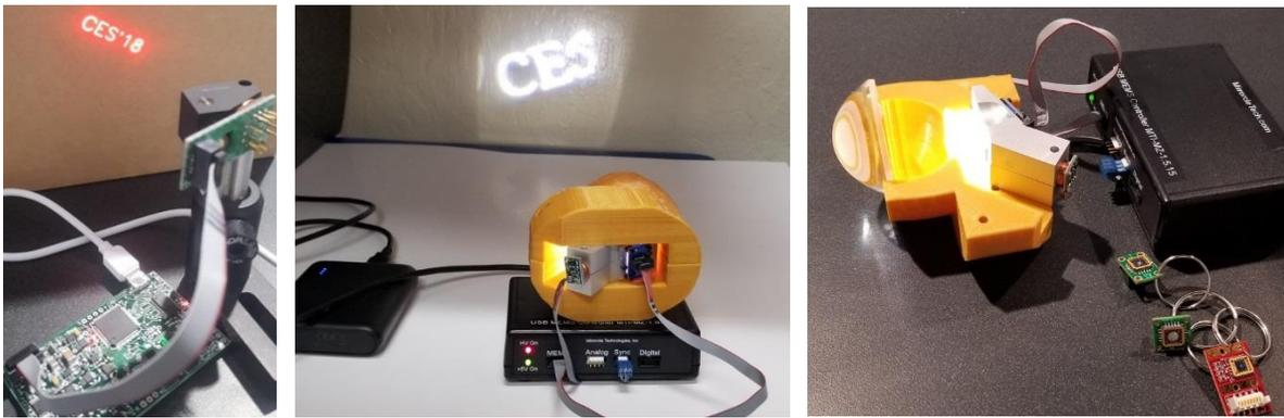
Figure 2. PLAYZER prototype with new USB Controller OCCIE 1.1 and new compact scan module (left). Programmable Light Source PLS-01 projecting white-light "CES" text (middle). Open PLS-01 module with MEMS-based scanner and integrated laser, phosphorous and optics. Also shown is the Mirrorcle USB-SL MZ controller powered by Microchip's PIC32MZ microcontroller (right).
